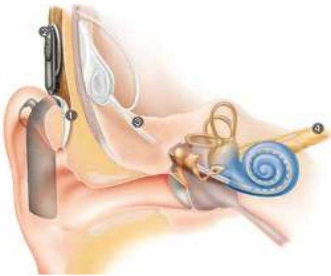
Figure 1. Schematic diagram of a cochlear implant (photo from Cochlear® website). Sound processor (1) worn behind the ear transmits digitally-coded sound through the coil (2) on the outside of the head to the implant. This then converts the digitally-coded sound to electrical impulses and sends them along the electrode (3) to the cochlea to directly stimulate the cochlear nerve (4).
